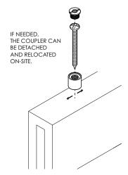
THE COUPLER CAN BE ATTACHED TO ANY 1/4"-20 THREADED SYSTEM. THIS INCLUDES A VARIETY OF CABLE GRIPPERS AND BOLTS.
